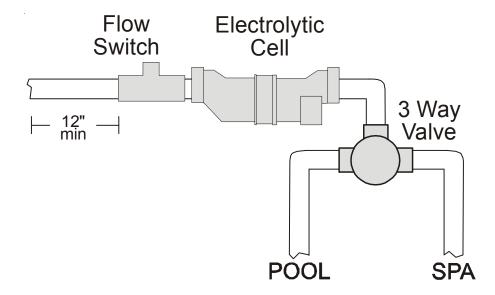
The cell may be mounted vertically or horizontally, and water can move in either direction through the cell. Install using the 2" unions provided. Tighten unions  $\underline{\mathbf{BY HAND}}$  for a watertight seal. For systems with  $1\frac{1}{2}$ " plumbing use adaptors (provided by installer).
