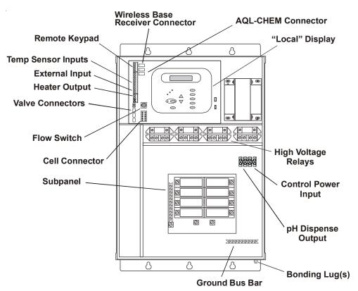
The Pro Logic Control Center requires both high and low voltage connections. Low voltage connections will be made to actuators, sensors, remote keypad, etc. High voltage connections will be made to pumps, lights, etc., as well as providing direct input power to the Control Center. Always:
