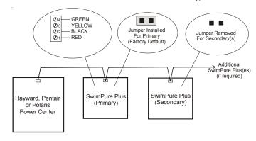
Hayward - Attach wires to proper screw terminals as shown below.
