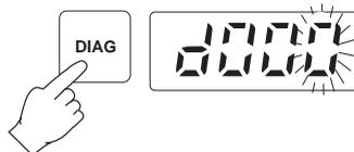
**Note** If the analyzer has been reset or turned on, “d000” will appear when pressing DIAG.
