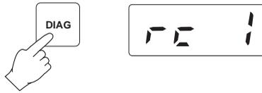
Microprocessor programming routines will measure and calibrate the output limits. This procedure will set the output to approximately 1% accuracy. Fine tune the recorder output by following the procedure in step 3.
