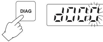
**Note** If the analyzer has been reset or turned on, "d000" will appear when pressing DIAG.
