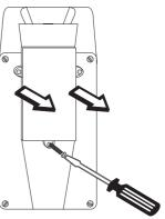
Make sure the battery contacts are tight and secure before replacing the cover.
