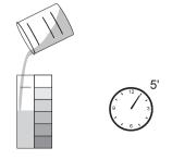
• Determine which color matches the solution in the cube, and record the results in mg/L (or ppm) NH<sub>2</sub>-N.
