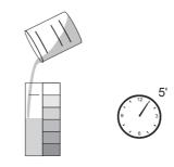
• Determine which color matches the solution in the cube, and record the results in mg/L (or ppm) NH<sub>a</sub>-N.
