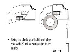
• Insert one of the vials into the left hand opening of the checker disc. This is the blank.
