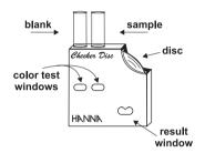
• Add to the other vial 1 packet of HI 93707-0 reagent. Replace the cap and mix to dissolve.
