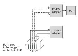
Note: It is recommended to terminate the line of the RS485 network, by plugging on the last HI142 the termination key supplied with the HI504903 supervisor, or connecting a resistor of about  $120\Omega$  as shown here below.
