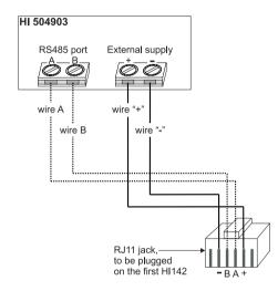
For connecting one **HI142** datalogger to the next one, make a cable as explained on the below diagram, by using a 4-wire cable and two RJ11 jacks (male connectors):
