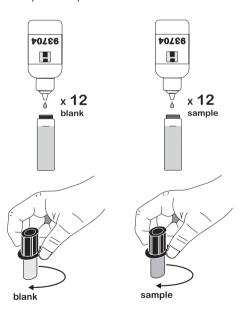
Place the blank into the holder and ensure that the notch on the cap is positioned securely into the groove.
