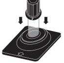
The mark on the cuvet cap should point towards the LCD.
