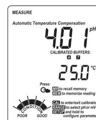
**Note:** During calibration, the secondary LCD shows the selected buffer value; press **RANGE** to display the buffer temperature.
