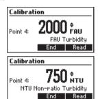
**Note:** If necessary, press **UP** or **DOWN** key to edit each calibration point value to match the exact value of the standard as measured with a reference turbidimeter.
