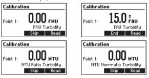
This point is used for FNU and NTU modes to check the quality of the water used for dilution and to confirm that the optical system is not dirty. In this case, if the value of the first point is over 0.15 FNU (NTU), a warning "Cal Point1 high!" is displayed when the calibration is saved and a warning "Out of calibration range" is displayed when measurements under 10.0 FNU (NTU) are performed.
