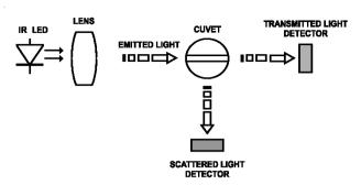
For the ratio turbidity mode, the microprocessor of the instrument calculates the NTU value, from the signals that reaches the two detectors, by using an effective algorithm. The optical system and measuring technique compensate the color interference and also the LED intensity fluctuations, minimizing the need of frequent calibration.
