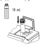
Press the Zero key. The display will show "-0.0-" when the meter is zeroed and ready for measurement.
