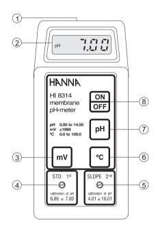
1) DIN connector for pH or ORP electrode
