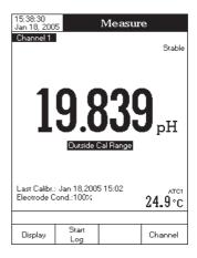
The pH reading is affected by temperature. In order to measure the pH accurately, the temperature effect must be compensated. To use the **Automatic Temperature Compensation** (ATC) feature, connect and submerge the **HI 7662-T** temperature probe into the sample as close as possible to the electrode and wait for a few seconds. If the temperature of the sample is known, **Manual Temperature Compensation** (MTC) can be performed by disconnecting the temperature probe.
