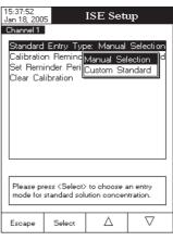
*Calibration Reminder* — See Calibration option from pH Setup section, page 20. *Set Reminder Period* — See Calibration option from pH Setup section, page 20. *Clear Calibration* — See Calibration option from pH Setup section, page 20.
