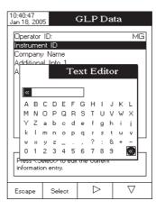
Press Escape to return to the GLP Data options. If the Saving Confirmation is enabled, press ves to accept the modified option, vo to escape without saving or cancel to return to the editing mode. Otherwise, the modified options are saved automatically.
