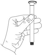
Using dropper provided, add about 2 mL of carbon dioxide internal fill solution HI 4005-40 into outer probe body.
