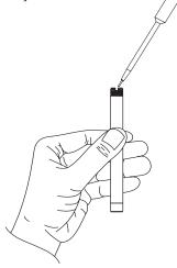
Insert and position the inner glass/reference assembly into the outer body so that the anti-rotation key sits in the cut out on the outer probe body.
