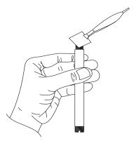
Hold one corner against the threads with thumb while gently stretching membrane over opening and capturing opposite membrane corner against threads . Smooth excess membrane material around the threads.
