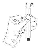
5.) Using dropper provided, add about 2 mL of ammonia internal electrolyte HI 4001-40 into outer probe body.
