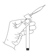
Screw outer membrane cap onto body thus capturing the membrane between the cap and outer body threads.
