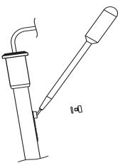
7. Holding the body of the electrode gently press upper cap with your thumb. This permits the fill solution to drain out of the body. Release cap and verify electrode returns to its original position. (You may need to gently assist for this to occur).
