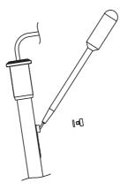
Holding the body of the electrode gently press upper cap with your thumb. This permits the fill solution to drain out of the body. Release cap and verify electrode returns to its original position. (You may need to gently assist for this to occur).
