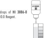
Determine which color best matches the solution in the cube and record the result as oH unit.
