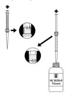
• Place syringe tip into the cap port of the plastic vessel and slowly add the titration solution drop by drop, swirling to mix after each drop. Continue adding titration solution until the solution in the plastic vessel turns colorless.
