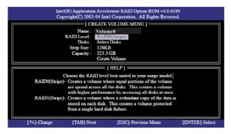
Use the up or down arrow keys to select your desired **RAID Level**. You may select RAID0 (Stripe), RAID1 (Mirror), RAID 5, RAID 10, or Matrix Storage for your RAID level. Press <Enter>, and then you can select **Strip Size**.
