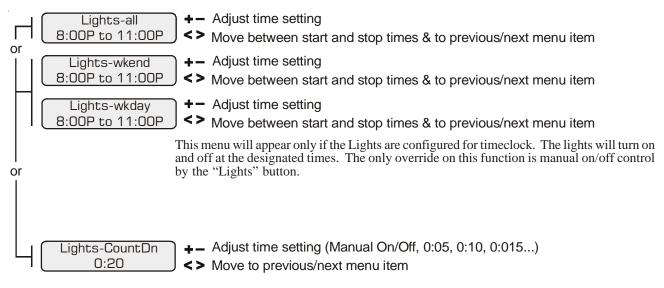
This menu will appear only if the Lights are configured for countdown timer. This setting is the time after you manually turn on the lights until the Pro Logic automatically turns off the lights. You can also manually turn off the lights at an earlier time by pressing the LIGHTS button. If the Lights relay is on during the programmed off time, it may be because of freeze protection.
