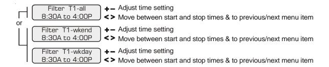
For one speed pumps, this is the first filter timeclock and will determine the normal hours of filtration for the pool. For pool/spa combination systems with spillover enabled, the valves will automatically switch to spillover mode at the start of the filtration period. For all other systems, the valves will switch to the pool-only position. Refer to the text above for general notes regarding timeclock programming.
