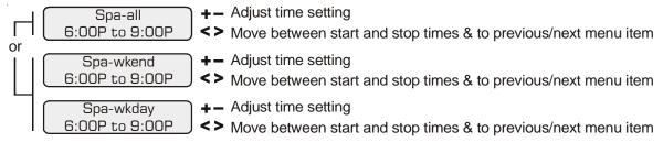
This menu is only available if the system has been setup for "pool and spa". During the programmed spa time, the Pro Logic will turn on the filter pump and move the pool/spa valves into the "spa-only" position. The heater will automatically heat the spa up to the programmed spa temperature (page 7). This programmed spa operation will take precedence over all other automatic functions, only manual operation of the filter button or pool/spa valve button will override this function.
