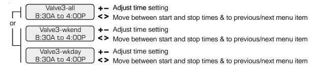
This menu will appear only if Valve3 is configured for timeclock. The valve will rotate on and off at the designated times. There is no manual override. If the Valve3 relay is on during the programmed off time, it may be because of freeze protection.
