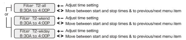
For one speed pumps, this is the second filter timeclock
