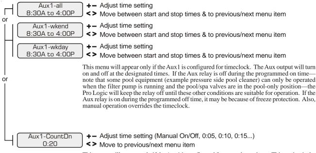
This menu will appear only if the Aux1 is configured for countdown timer. This setting is the time after you manually turn on the Aux relay until the Pro Logic automatically turns off the relay. You can also manually turn off the relay at an earlier time by pressing the AUX1 button.
