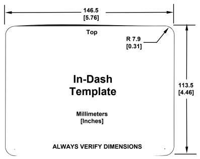
In-dash mounting template for the GlobalMap 5200c, showing dimensions. NOTE: The figure above is *not* printed to scale. A scaled template (FM-5 In-Dash Adapter Kit instructions) is available for free download from our web site, www.lowrance.com.
