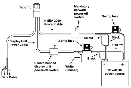
Use this method if you are powering the display unit and a GPS module or the display unit and a NMEA 2000 network. (Fuses may be different from those shown.).
