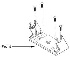
Install the gimbal bracket. Orient the bracket so the arms slope toward the front of your unit.
