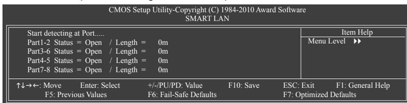
This motherboard incorporates cable diagnostic feature designed to detect the status of the attached LAN cable. This feature will detect cabling issue and report the approximate distance to the fault or short
