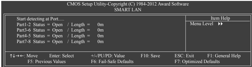
This motherboard incorporates cable diagnostic feature designed to detect the status of the attached LAN cable. This feature will detect cabling issue and report the approximate distance to the fault or short.
