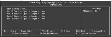
This motherboard incorporates cable diagnostic feature designed to detect the status of the attached LAN cable. This feature will detect cabling issue and report the approximate distance to the fault or short.
