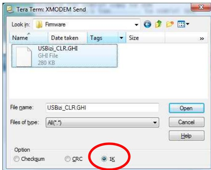
Updating the firmware takes a few seconds to load. Once loading has finished and the file is valid, the new firmware is executed automatically and you will not see “BL” again.
