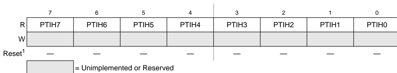
Figure 22-49. Port H Input Register (PTIH)
