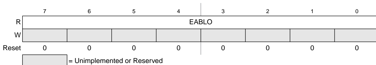
Figure 25-14. EEPROM Address Low Register (EADDRLO)
