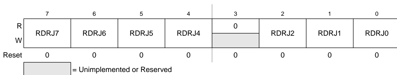
Figure 23-59. Port J Reduced Drive Register (RDRJ)
