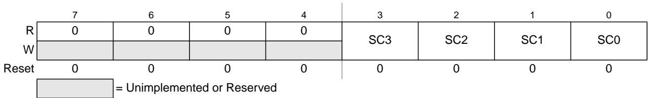
Figure 20-9. Debug State Control Register 1 (DBGSCR1)
