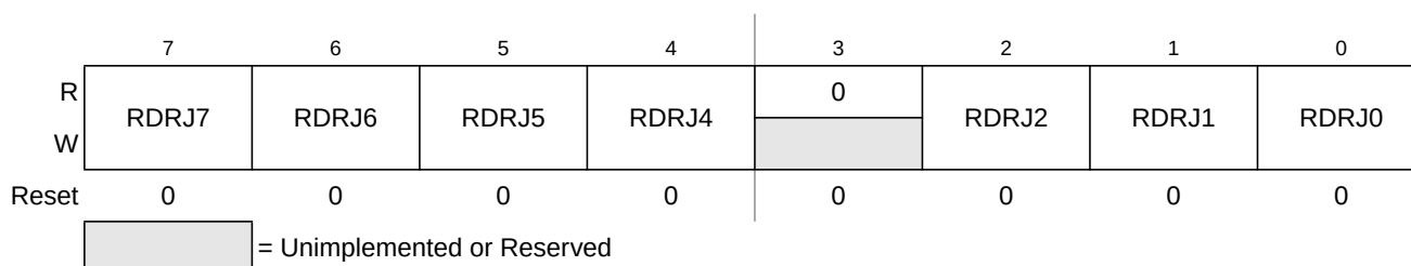
Figure 22-59. Port J Reduced Drive Register (RDRJ)
