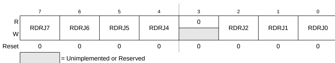
Figure 23-59. Port J Reduced Drive Register (RDRJ)
