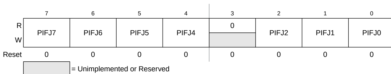
Figure 22-63. Port J Interrupt Flag Register (PIFJ)
