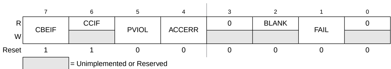
Figure 27-13. Flash Status Register (FSTAT — Special Mode)
