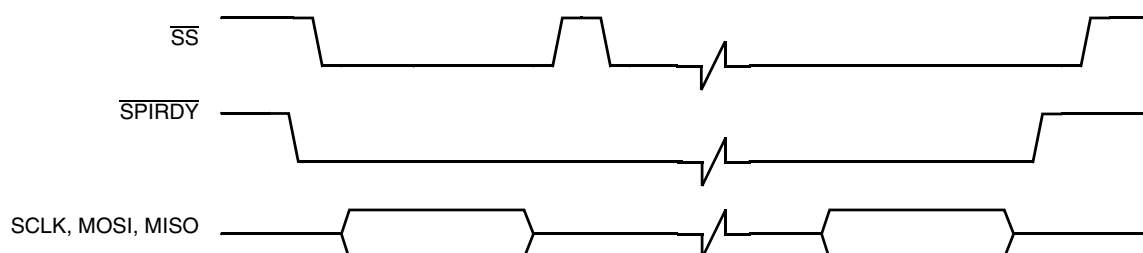
Figure 15. Master SPI Timing Diagram Using \overline{\text{SPI\_RDY}} Level Trigger
