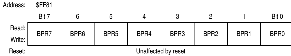
Figure 2-8. FLASH-2 Block Protect Register (FL2BPR)
