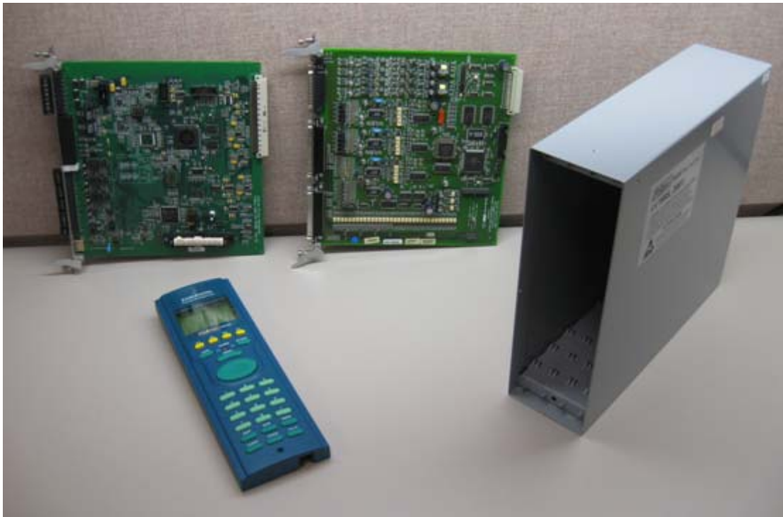
Figure 2-1. FloBoss S600+ System Components
