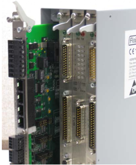
Figure 2-10. Module Ready for Removal or Insertion
