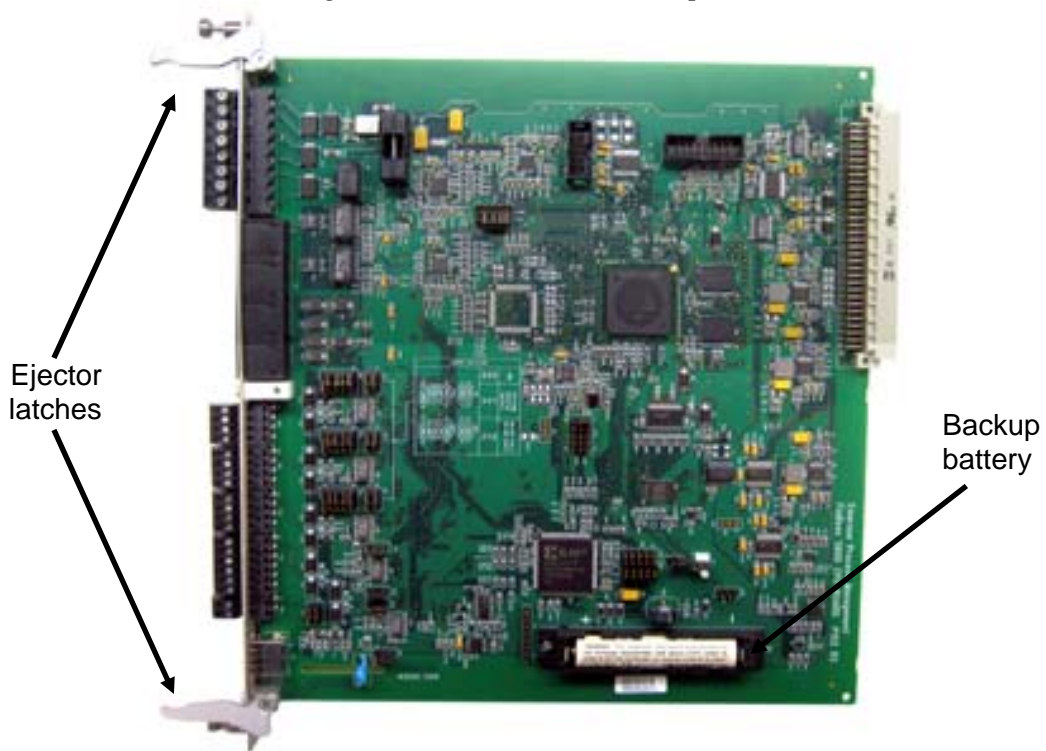
Figure 3-1. CPU Module Backplate
