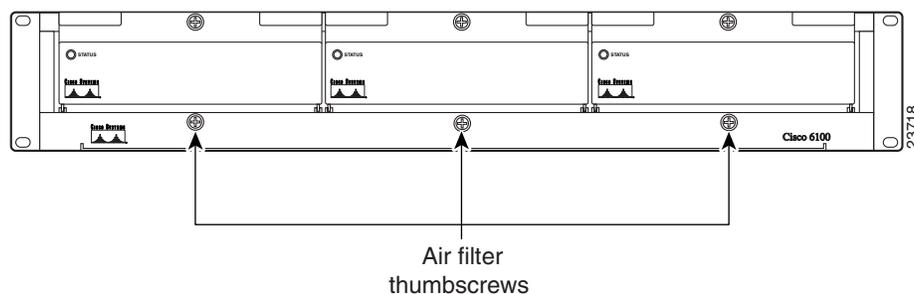
**Step 3** Carefully remove the air filter door.
