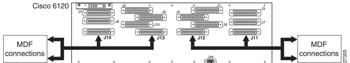
Figure B-10 shows the cabling between the voice lines on the Cisco 6120 and the voice-switching equipment that provides local POTS service. The cables listed in Table B-5 are used for the connection.
