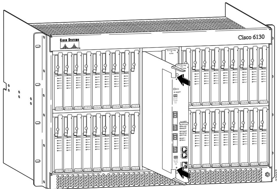
**Step 4** Lift up on the locking levers and gently apply pressure to the bottom of the faceplate while pushing the card into the slot.
