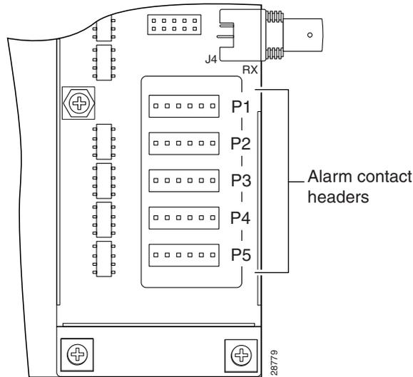
Table 3-3 maps the wire-wrap pins to the alarms that are supported by the NI-2 card through the Cisco 6130 backplane.
