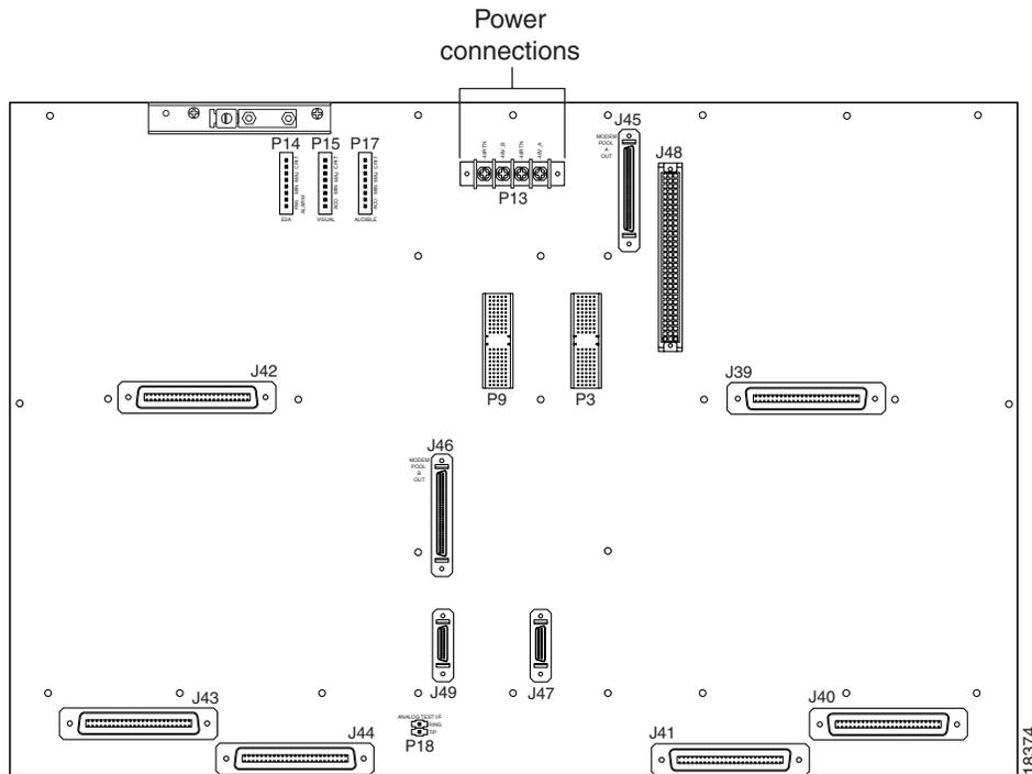
You can wire the power connections from the Cisco 6130 to the fuse and alarm panel for either dual- or single-power feed:
