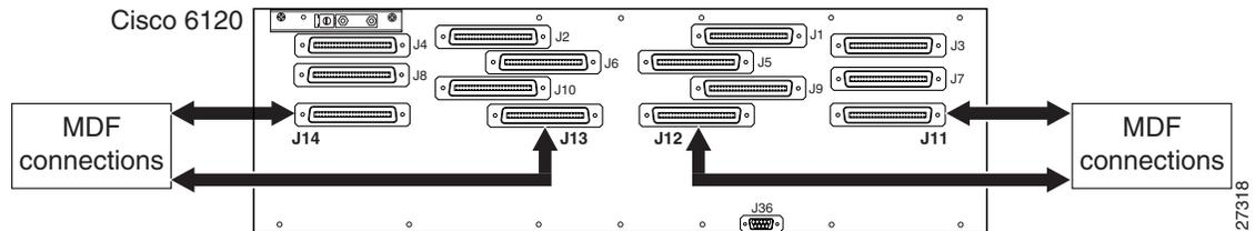
Figure B-7 shows the cabling between the Cisco 6120 to the POTS service connections in which the cables listed in Table B-4 are used.
