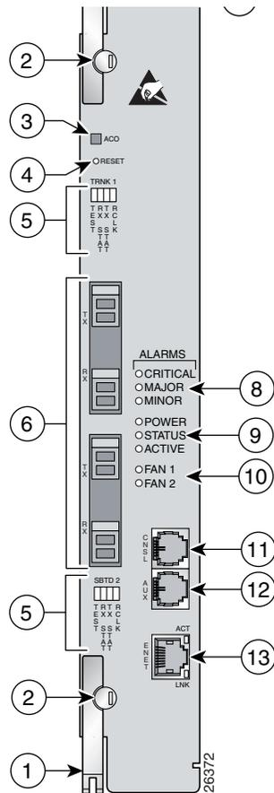
The transmit connector is the one closest to the top of the faceplate. The receive connector is closest to the bottom of the faceplate. The connector IDs are silkscreened inside the inset.
