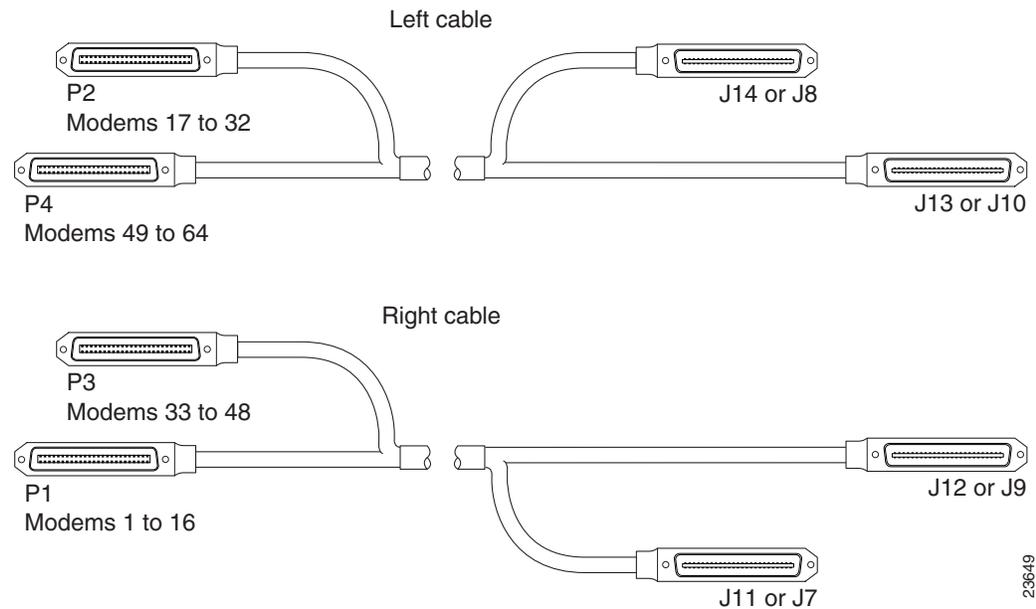
Figure B-9 shows the cabling between the xDSL subscriber line connectors on the Cisco 6120 and the MDF in which the cables listed in Table B-5 are used.
