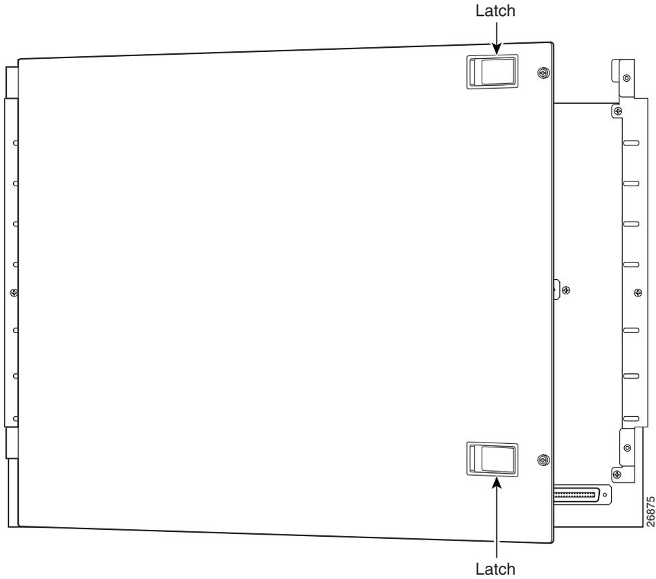
**Step 2** Release the latches after the rear cover is in place.
