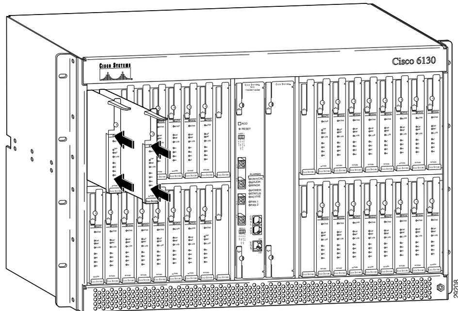
**Step 6** Push on the faceplate of each line card to fully seat the line card.
