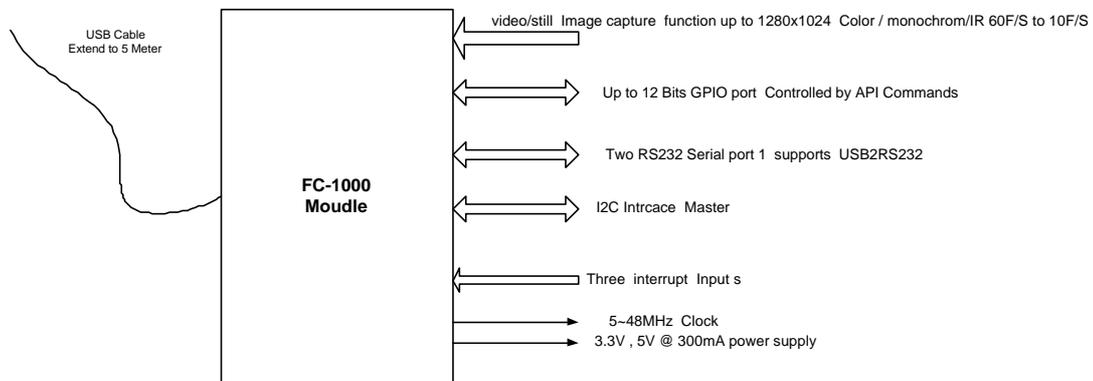
FC-1000 USB2 Camera Moudle Hardware Resource Block Diagram
