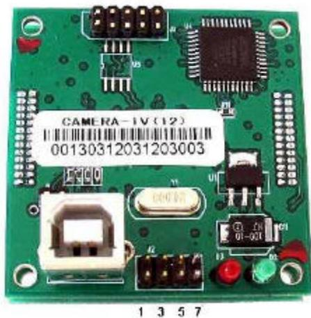
J2 Pin 1 Strobe signal : 3.3V. Active. During exposure this signal will change to high to turn on a possible lighting device such as flash tube, LED bar. This signal can be use for capture a high speed moving object that ignore Rolling shutter weakness.
