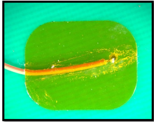
Figure 5: A 36 gauge thermocouple with polyimide tape as suggested for testing.
