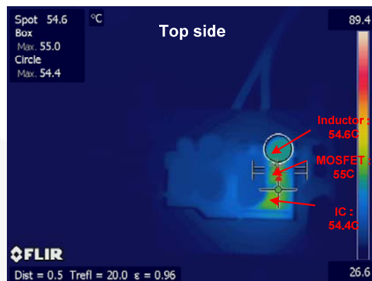
Figure 35. Thermal Test Result, Top-Side Temperature at 220V AC Condition (Inductor)
