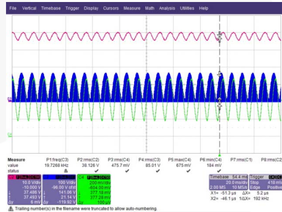
Figure 16. Input Voltage: 110V AC , Input Frequency: 64Hz, CH2: V OUT , CH3: V DRAIN , CH4: I LED
