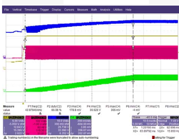
Figure 10. Soft-Start, DC Mode, 100V DC CH1: V CC , CH2: V DRAIN , CH3: V LED , CH4: I LED
