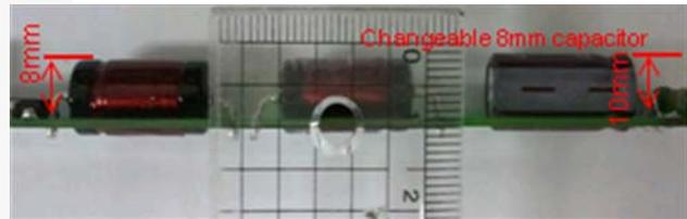
**Figure 4. Height: 10mm (Include PCB Height)**
