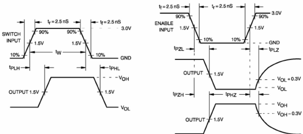
Figure 4. AC Waveforms
