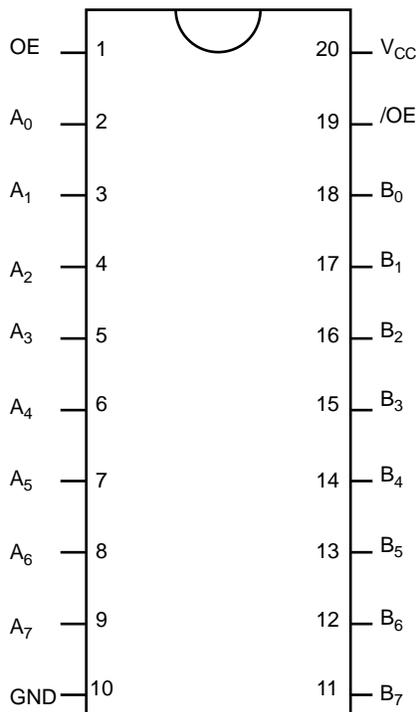
Figure 2. Pin Configuration
