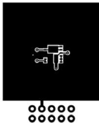
a. 65\text{ }^{\circ}\text{C/W} when mounted on a 1\text{ in}^2 pad of 2 oz copper, the board designed Q1+Q3 or Q2+Q4.
