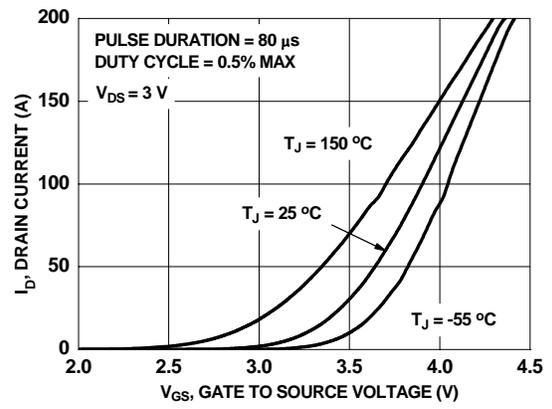
Figure 5. Transfer Characteristics
