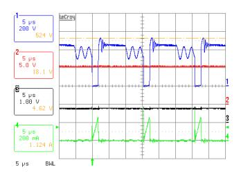
Figure 7. Steady-State Waveforms with 10nF Snubber Capacitor and  $14k\Omega$  Snubber Resistor
