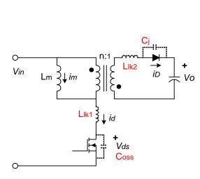
(a) Configuration with parasitic components
