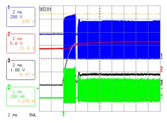
Figure 4. Start-up Waveforms with 1nF Snubber Capacitor and  $480 k\Omega$  Snubber Resistor
