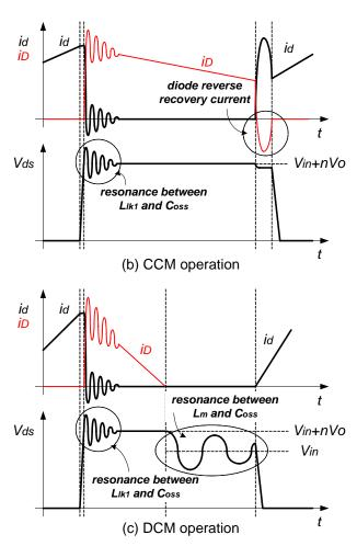
Figure 1. Flyback Converter; (a) Configuration with Parasitic Components, (b) CCM Operation, (c) DCM Operation
