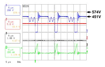
Figure 5. Steady-State Waveforms with 1nF Snubber Capacitor and 480kΩ Snubber Resistor
