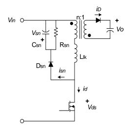
Figure 2. Flyback Converter with RCD Snubber
