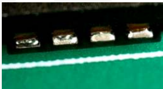
Figure 2. Exposed Copper on Package Edge, Solder Wetting after Reflow, Singulation Process
