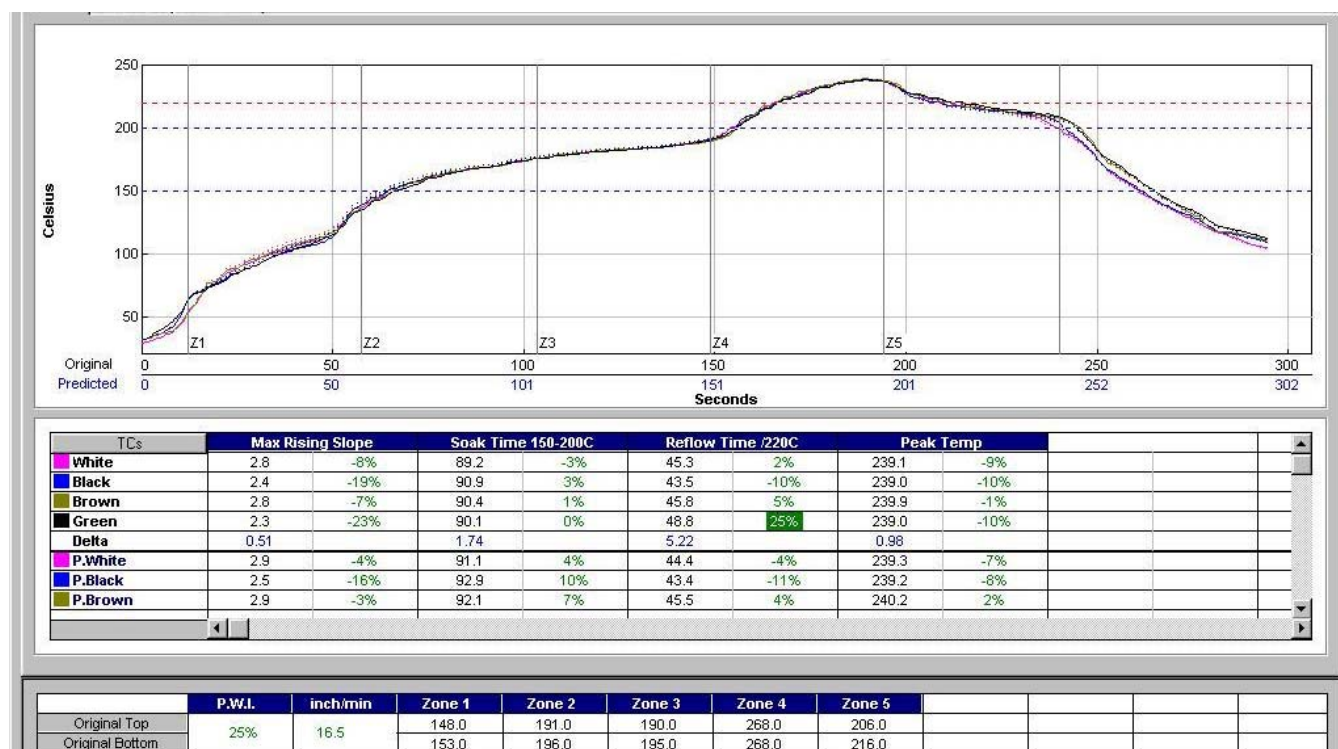
Figure 5. Reflow Profile used for Building Demonstration Boards
