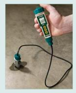
Extension cable and weight attached to meter and electrode module for easy measurement on concrete
